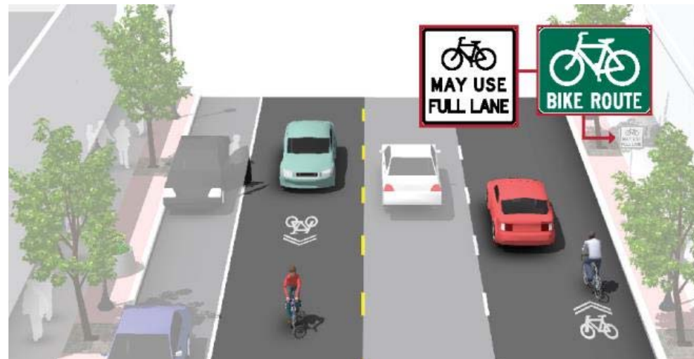
Example of a Shared Roadway using shared lane markings and signage. Source: NACTO
