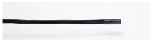
Epoxy tip with parallel 24 gage, PVC insulated leads (parallel bonded). For general purpose temperature measurement. Not for continuous immersion in water (mineral or silicon oil is OK).
