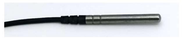
Rugged stainless steel probe 6 mm (0.236") diameter and 50 mm (approx 2 inch) length with 6.1 meter (20 ft) cable. TPE jacketed cable has diameter of 3.3 mm (0.13"), round cross section and 24 gage, polypropylene insulated leads. Suitable for immersion, HVAC, and soil burial applications. Probe's cable not recommended for immersion in fuels (fuel splashing on cable is OK).
